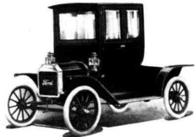
2-Passenger Coupe, Equipped with 3 Oil Lamps, Tubular Horn and Kit of Tools
