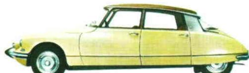
With options - front and rear optional bars, tinted windows, sun visors, ground clearance indicator, electronic equipment, the last model of the ID 19 is equipped with the DS 21. The DS 21 has a 1.9 liter engine, 100 bhp, 4-speed transmission, 4-wheel disc brakes, power steering, power brakes, front wheel drive, and a top speed of 120 km/h (75 mph). Weight: 1,250 kg (2,765 lbs). Price: 1,250,000 francs.
